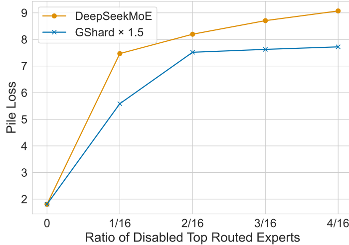
Figure 4 | Pile loss with regard to different ratios of disabled top routed experts. Notably, DeepSeekMoE exhibits greater sensitivity to the ratio of disabled top routed experts, indicating lower redundancy among routed experts in DeepSeekMoE.
